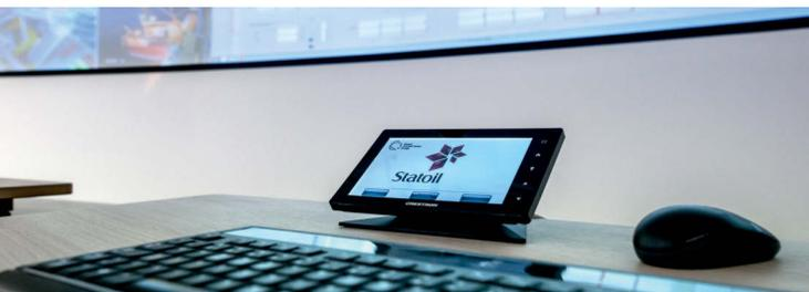
**A powerful Crestron Control System operated from a Crestron Touch Panel controls six projectors and a RGB Spectrum Mediawall (photo: GCCD)**
